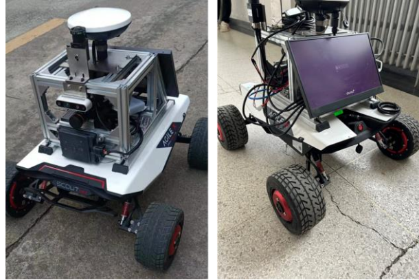
Fig.2 Configuration of modified UGV as experimental platform
