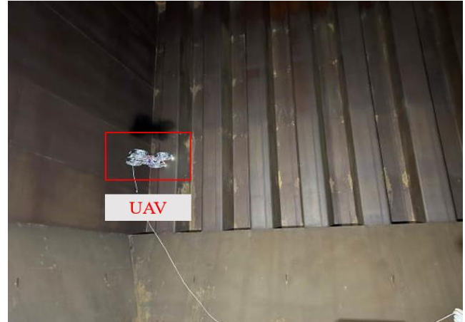
Fig.4 UAV flight test scenario inside the tanker hold.
