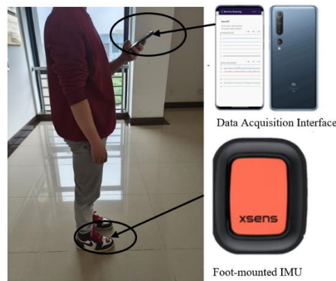
Fig.3 IMU Wearing Styles and Data Acquisition Interface
