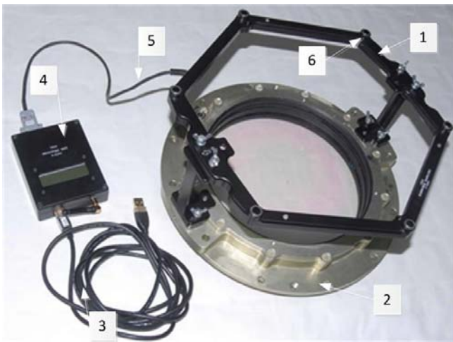
Fig. 2. Receiver platform with control unit: 1 – platform located around the window, with ultrasonic receivers; 2 – porthole; 3 – cable connecting the control unit to the crew computer; 4 - control unit with Wi-Fi communication device; 5 - cable for connecting ultrasonic receivers to the control unit; 6 – ultrasonic receiver.
