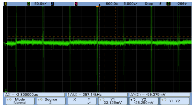
Fig. 5. Test results of power supply interference at the PIN-FET end of the gyroscope after filtering
