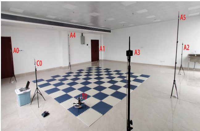
Fig. 6. Schematic diagram of the layout of the UWB positioning system for indoor environment experiments
