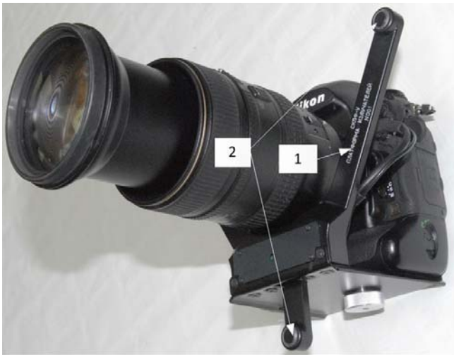
Fig. 1. Photocamera with a platform of emitters: 1 – platform attached to the camera; 2 – ultrasonic emitters.
