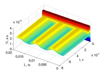
Fig. 6. Population inversion grating during lock-in of counterpropagating waves
