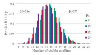
Fig. 1. Probability distribution of the number of visible satellites for two users with roll ( $\beta_1$ =20°,  $\Delta L$ =0 km)
