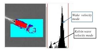
Detection of the aircraft carrier escort ship by its wake
