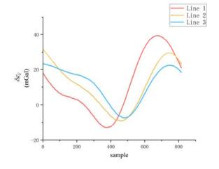
Fig. 6. Measurement results of the eastern component of gravity disturbance based on SINS/GNSS
