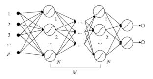
Fig. 2. Neural network architecture (M – the number of hidden layers, N – the number of neurons)
