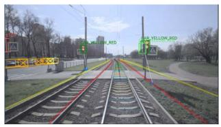
Figure 4. Fragments of visualization of traffic lights recognition results
