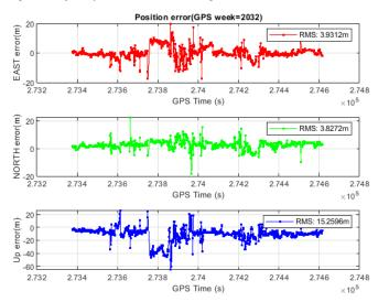
Fig. 2. The position errors in three directions with usual KF
