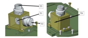
Fig. 6. Thermocouples mounting on the accelerometer bracket
