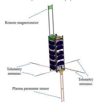
Fig. 1. SamSat-ION NS in the flight configuration
