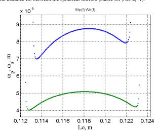
Fig. 9. Beam sizes in the gain medium for the plane of incidence on the mirror  $\omega_p$  (top) and in the perpendicular plane  $\omega_s$  (bottom) when changing the distance Lo between the spherical mirrors.
