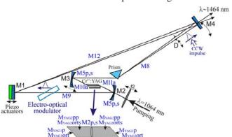
Fig. 7. Optical scheme of an astigmatic ring cavity for Kerr mode-locking.
