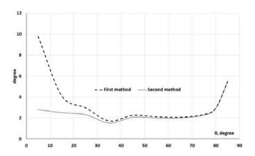
Fig. 2. Azimuth estimation errors as functions of the elevation angle under  $\phi=56.8^\circ,\, A=45^\circ,\, \psi=0^\circ$
