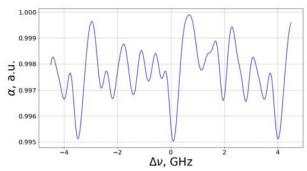
Fig. 18. Dependence of the transmittance  $\alpha$  of an acetylene cell on the laser frequency tuning  $\Delta\nu$  during multifrequency lasing. The linewidth of the absorption maximum is ~250 MHz (line near  $\Delta\nu$ ~0).
