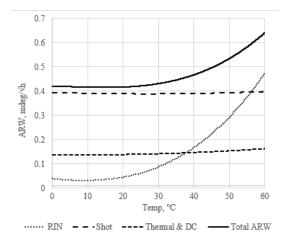
Fig. 3. Dependence of ARW components on temperature
