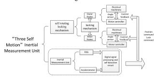
Fig. 1. "Three self motion" Inertial Measurement Unit Composition Block Diagram
