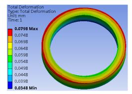
Fig. 4. Simulation result of fiber coil deformation
