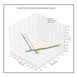
Fig. 4. Comparison of measured, estimated and reference trajectories
