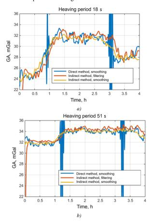
Fig. 2. Estimates for the vertical component of the accelerometer bias by using the direct method (smoothing) and indirect method (filtering and smoothing) a) heave period 18 s; b) heave period 51 s.
