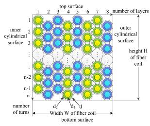
Fig. 2. Rectangular cross section of fiber coil wound with 8-pole symmetrical method
