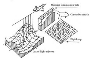
Fig. 7. Terrain Matching Diagram of UAV [15]
