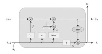
Fig. 3. LSTM ANN cell architecture, here  $X_t$  is the input time step,  $h_t$  is the output,  $C_t$  is the cell state,  $f_t$  is the forget gate,  $i_t$  is the input gate,  $o_t$  is the output gate,  $\hat{C}_t$  is the internal cell state. Operations inside dark grey circle are pointwise.
