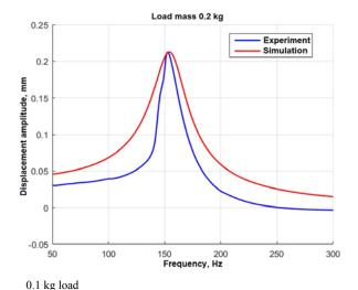
Fig. 3. Comparison of model and experimental shock absorber AFR under  $0.2~\mathrm{kg}$  load
