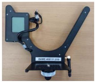
Fig. 3. Emitter platform with a small-sized screen.
