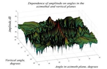
Fig. 2. Dependence of amplitude on angles in the azimuthal/vertical planes
