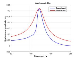
Fig. 4. Comparison of model and experimental shock absorber AFR under 0.3 kg load
