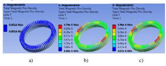
Fig. 8. Simulation results of radial magnetic field: a) Magnetic induction intensity without magnetic shielding, b) Magnetic induction intensity during single-layer magnetic shielding, c) Magnetic induction intensity during double-layer magnetic shielding.
