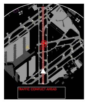
Fig. 3. Cockpit screen with active SURF IA.
