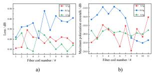
Fig. 4. Fiber coils with different coiling tensile forces: a) the loss, b) the maximum polarization crosstalk
