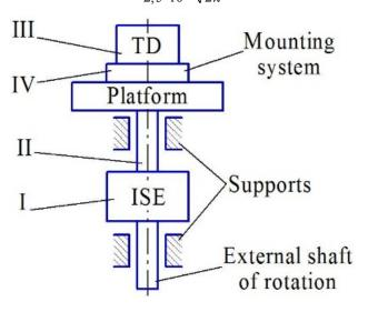
Fig. 2. Main elements in the bench structure affecting its accuracy characteristics
