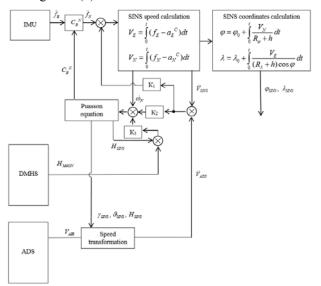
Fig. 9. Navigation complex algorithm
