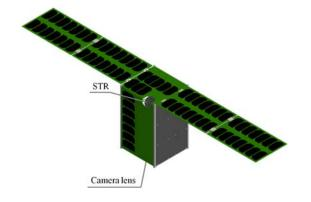
Fig. 1. STR installation in the satellite
