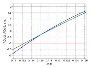
Fig. 8. Stability parameters for p (*blue*) and s (*green*) planes when changing the distance Lo between the spherical mirrors (stable for |AD/2|<1).
