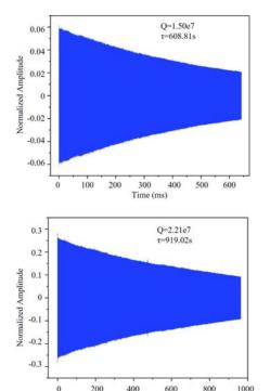
Fig. 3. The measured ring-down curve of different resonators showing its ultra-high Q factor of 15 million and 22 million.
