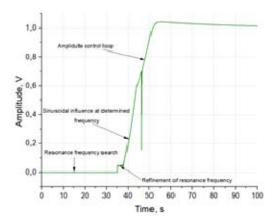
Fig. 4 The Oscillation amplitude change when using rhe existing actuation algorithm
