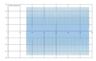
Fig. 3. Heading angle during rotation with accleration 0.2g
