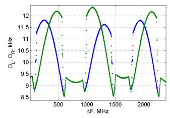
Fig. 5. Dependence of the bias of the beats of orthogonal polarizations Asin and Bsin on lasing frequency tuning by piezo motors. The signal separation was performed by an electronic system.
