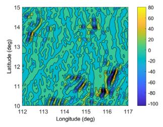
Fig. 1. Calculation results of disturbance gravity gradient  $T_{xx}$  component
