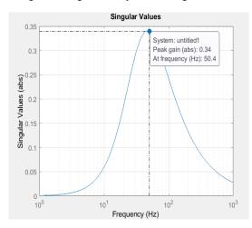
Fig. 6. Changes in the singular value of the closed system
