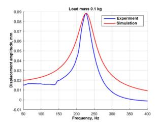
Fig. 2. Comparison of model and experimental shock absorber AFR under
