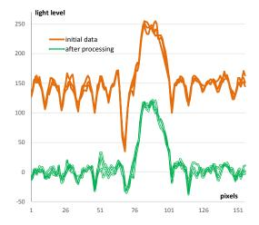
Fig. 4. Separation of the laser module light line before and after primary processing
