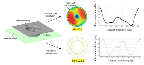
Fig. 1. A 300 K temperature fluctuation at 3mm depth indicated by fluid-structure interaction (FSI) analysis, and a similar distribution of circularity error measured on a fabricated resonator at the same position
