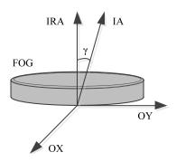
Fig. 1. Schematic diagram of input axis misalignment angle
