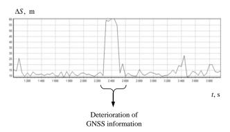
Fig. 3. Circular error of estimating the location of the RPA in the inertial-satellite mode
