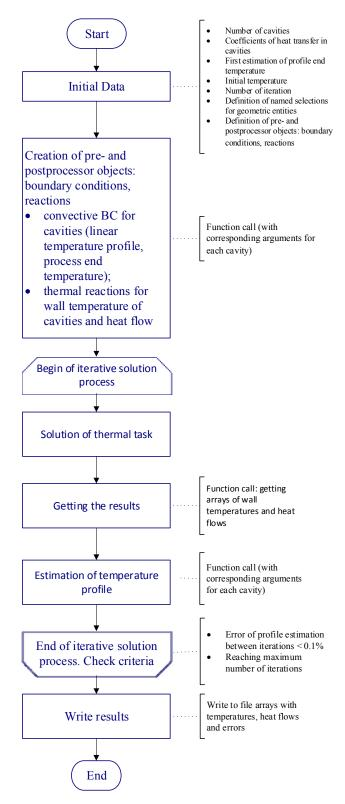
Fig. 1. Algorithm of the calculation technique
