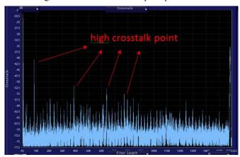
Fig. 2. Distributions of crosstalk points in a PM fiber coil
