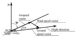
Fig. 7. Drift angle without sideslip.
