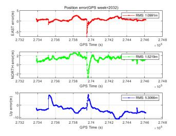
Fig. 4. The position errors in three directions with adaptive MCC based robust CKF
