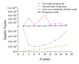
Fig.5. Effect of anchor height h on the quality factors of the hemispherical resonators
