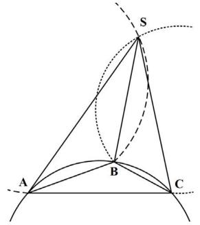
Fig. 2. Geometric chart showing how to determine position of point S from the known positions of points A, B and C
