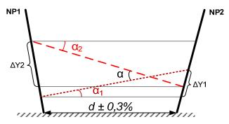
Fig. 2. Change in the mutual angular position of NP1 and NP2 in the longitudinal plane
