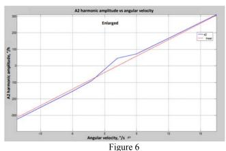
The linearity upsets only at low angular velocities  $\omega$  < 5°/s. At the rest velocities the deviation from linearity is not higher than 20 °/h.
