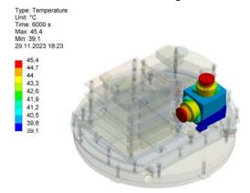
Fig. 8. Temperature field in the accelerometer bracket
