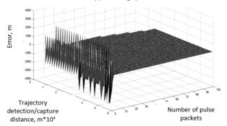
Fig. 1. Errors of active AR tracking in range in the presence of anomalous estimates at the stage of detecting/capturing the target trajectory
