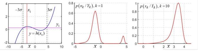
Fig. 1. Nonlinear function of measurements and a posteriori PDF for k = 1 and k = 10.
