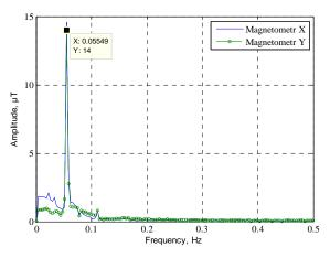
Fig. 4. Spectral characteristics of magnetometric sensors
