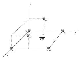
Fig. 1. Schematic diagram of system layout
