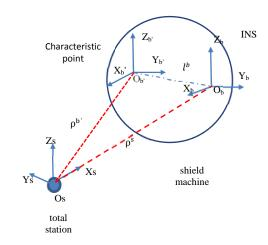
Fig. 1. Equipment installation relationship and the definition of the main coordinate systems  $Z_s$
