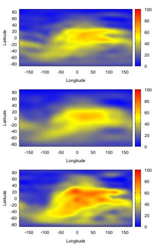
Fig. 2. TEC map built on the basis of an autoregressive model for expansion up to degree 15 (top) to degree 9 (in the center) and the original TEC map from CODE at 12:00 UTC January 10, 2024 (bottom).
