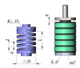
Fig. 2. An elastic element and a nonlinear dynamic vibration damper, where  $K_1$  and k are the elasticity coefficients;  $D_1$  and d are damping coefficients; h is a gap;  $m_2$  is the mass of blocks; t, a, L are spring parameters.
