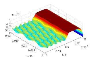
Fig. 4. Population inversion grating in beat mode. The beat frequency is determined by frequency nonreciprocity.
