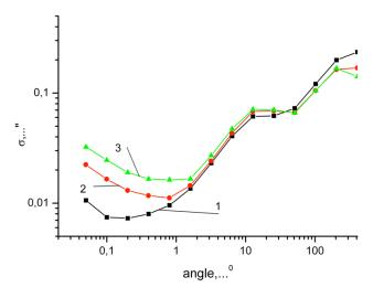
Fig. 1. Allan variances depending on the angle of rotation at rotation speeds: 1-0.2 22 rad/s; 2-3 22 rad/s; 3-5.6 22 rad/s
