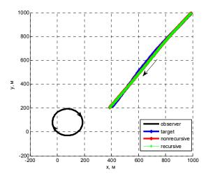
Fig. 2. Coordinate estimates for the nonrecursive iterative linearized batch smoother and recursive iterative linearized Kalman smoother.
