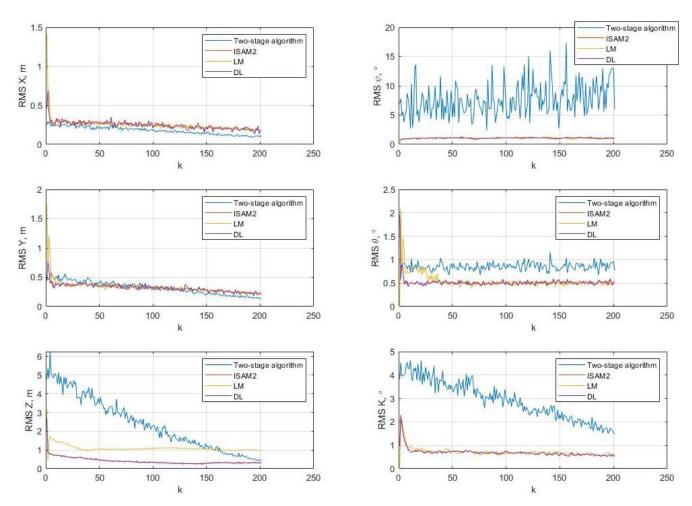
Fig. 2. Dependence of the RMS of the AUV coordinates and orientation angles on the moments of time k.
