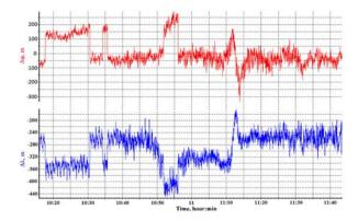
Fig. 10. LRNAV coordinate measurement errors.
