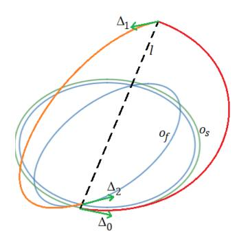
Fig. 1. Schematic of a 3-pulse maneuver. Here  $o_s$  – start orbit,  $o_f$  – finish orbit, l – line of nodes,  $\Delta_0$  – first maneuver impulse, taking the spacecraft from the orbit of the first debris,  $\Delta_1$  – second impulse, turning the orbit plane,  $\Delta_2$  – third impulse, equalizing the spacecraft speed with the speed of the second debris, two elliptical pieces of the flight path between the debris are shown in red and orange.
