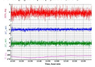
Fig. 8. DNS parameter errors in the flight segment.
