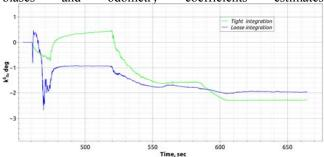
**Fig. 5.** Estimate of  $k_0^{\delta}$  zero offset of the steering angle sensor
