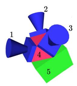
Fig.1. The layout of the strapdown AINS. 1,2,3-AVU cameras; 4-AVU base; 5-IMU;
