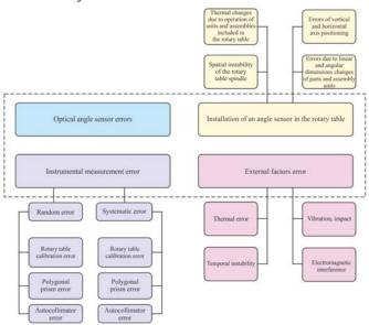
Fig. 1. Rotary table error model.
