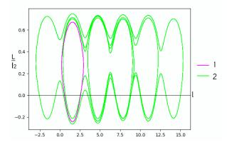
Fig. 4. Phase trajectories, 1 - unperturbed motion, 2 - perturbed motion
