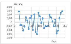
Fig. 4. The sum of the random errors of the MIU and LIR sensors
