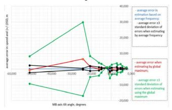
Fig. 4. Average values and ±3SD intervals for speed determination errors based on the average frequency and global maximum
