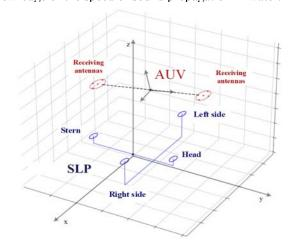
Fig. 1. Layout of AUV hydroacoustic system and SLP.
