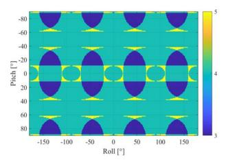
Fig. 7. Number of sensors registering the IR radiation at different attitudes of the nanosatellite relative to the Earth
