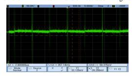
Fig.5 Test results of power supply interference at the PIN-FET end of the gyroscope after filtering
