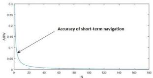
Fig.1. Graph of Angle Random Walk (ARW) dependence on the number of measuring modules (N) at ARW = 0.3 7 Vh
