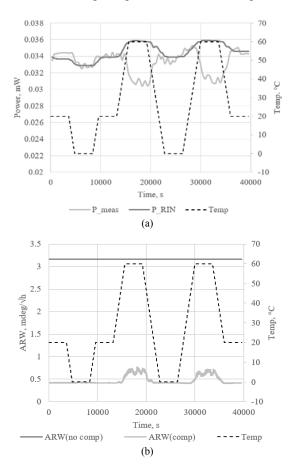
Fig. 2. Graphical results of the experiment on measuring the temperature dependence of (a) output powers of the arms of the VOG circuit with RIN compensation and (b) calculated value of ARW
