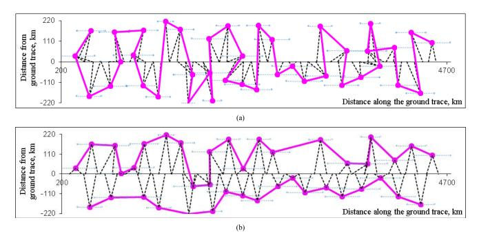
Fig. 4. Optimized sequences of object observation with minimum 20 sec time of object visibility from the SC 400 km orbit: (a) -  $\Delta$ =12 s, K=1; (b) -  $\Delta$ =20 s, K=2 ( $\Delta$  – minimum guaranteed shooting time for each object; K – number of parallel shooting processes).
