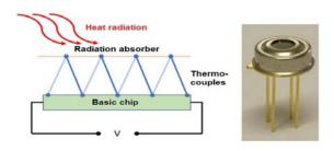
Fig. 1. Diagram of the thermopile structure (right) and photo of IR sensor model (left)
