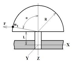
Fig. 1. Typical resonator-base connection in HRGs
