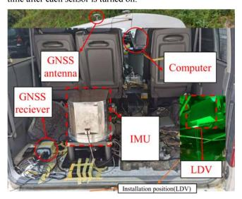
Fig. 3. Installation diagram of experimental equipment
