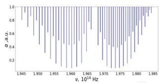
Fig. 17. Acetylene absorption spectrum in the region of 1.5 µm.
