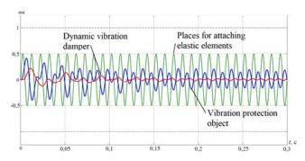
Fig. 6. Results of modeling the movements of the damping system at  $\Delta x_2 < h/2$ .
