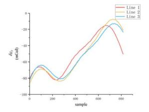
Fig. 10. Measurement results of the northern component of gravity disturbance based on SINS/GNSS/LDV
