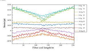
Fig. 6. Stress analysis curve of fiber coils with different coiling tensile forces at different temperature
