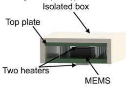
Fig. 5. AHRS NV-1 temperature stabilization system
