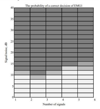
Fig. 1. The probability of correctly determining of the SS subspace dimension
