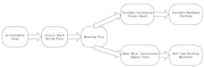
Fig. 9. Accuracy Traceability Flowchart.
