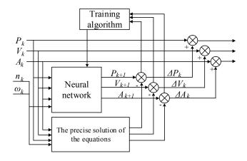
Fig. 1. Block diagram of the INS ideal operation algorithm approximation by the ANN
