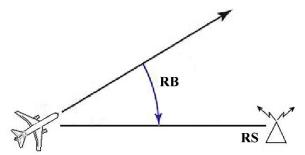
Fig. 1. Relative bearing of radio station.
