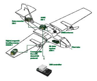
Fig. 3. Navigation complex for UAV
