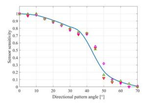
Fig. 4. Comparison of experimental and standard SDP
