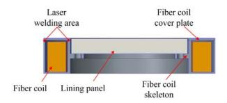
Fig. 4. Single-layer magnetic shielding structure
