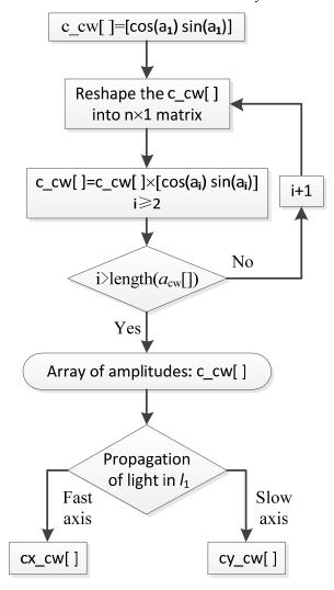
Fig. 3. Flow chart of amplitude calculation
