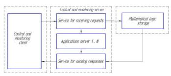
Fig. 3. "Control client and server" structural diagram.
