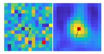
Fig.2. Motion blur correction in the image of a single star, observed against the background of the daytime sky. On the left is an image of a star taken in the single frame. On the right is the result of accumulating of 40 consecutive frames with the star's images. The black spot is the starting point of the blur trajectory, the black line is the blur trajectory, the red square is the brightest pixel of the image.
