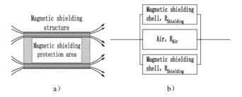
Fig. 3. Magnetic Shielding Principle: a)Structure Diagram of Magnetic Shielding Principle; b) Equivalent Magnetic Circuit
