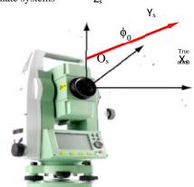
Fig. 2. total station measurement coordinate system (s system)
