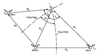
Fig. 9. Aircraft position determination using LRNAV stations
