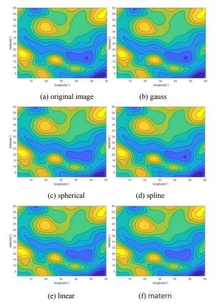
Fig. 2. The original function image and the kriging interpolation results using different kernel function types.
