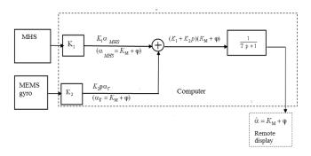
Fig. 1. Block diagram of the magnetic compass correction system based on a complementary filter.
