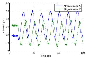
Fig. 2. Output signals of magnetometers on a rotating base
