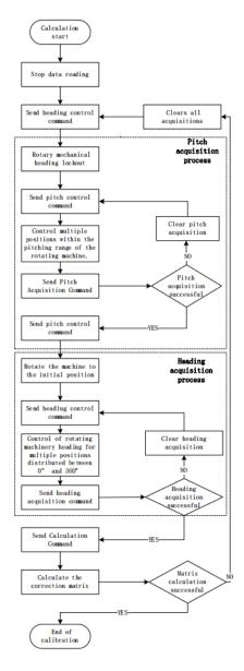
Fig. 5. Schematic diagram of the computational flow of the algorithm.
