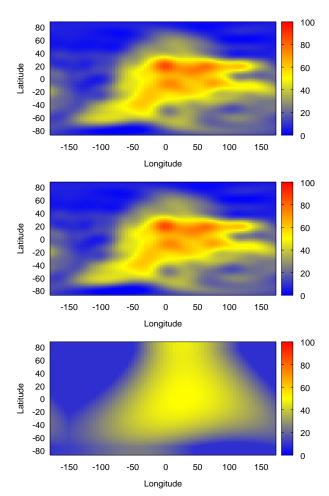
Fig. 1. An example of a global TEC map reconstructed from spherical expansion coefficients up to degree 15 (top). The original map from the IAC PNT is in the center. Below is a TEC map constructed based on the Klobuchar model by the Astronomical Institute of the University of Bern. The maps represent the spatial distribution of TEC in TECU at 12:00 UTC on January 10, 2024.)
