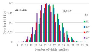
Fig. 3. Probability distribution of the number of visible satellites for two users with roll ( $\beta_1$ =10°,  $\Delta L$ =50 km)
