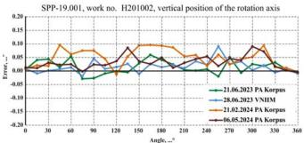
Fig. 4 Graphs of errors of two rotary tables obtained for one year of observation.
