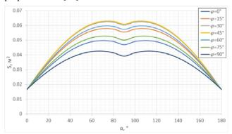
Fig. 2. Projection area of the SamSat-ION NS onto a plane perpendicular to the oncoming flow
