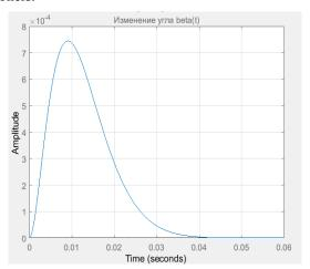
Fig. 4. Changes in the angle of rotation of the sensing element
