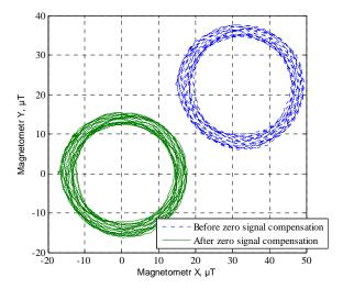
Fig. 3. Elimination of offsets of zero signals
