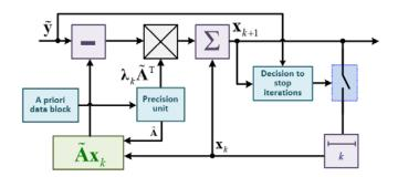
Fig. 2. Structural diagram of the algorithm of simultaneous algebraic reconstruction with input constraints
