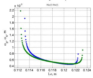
Fig. 10. Beam size on the output mirror for the plane of incidence on the mirror  $\omega_p$  (*blue*) and in the perpendicular plane  $\omega_s$  (*green*) when changing the distance Lo between the spherical mirrors.
