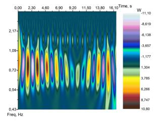
Fig. 3 The wavelet spectrum of an array of random variables characterizing a random error at a rotational speed of  $3\,\text{\ensuremath{\mathbb{Z}}}$  rad/s
