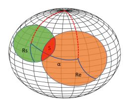
Fig. 2. Projections of sensor's field of view and the Earth on a unit sphere.
