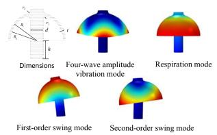
Fig.3. Dimensions and main mode shapes of the hemispherical resonator.
