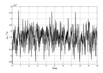
Fig. 5. Instability of the bench angular rate under simultaneous action of errors  $M_a$ ,  $\Delta U_m$ ,  $M_\beta$ ,  $\Delta U_{fog}$  and  $M_\phi$  (in the case of aerostatic supports and shock absorber node application).
