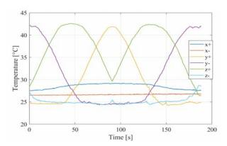
Fig. 9. Readings of IR sensors during bench tests
