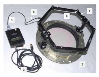
Fig. 2. Receiver platform with control unit: 1 – platform located around the window, with ultrasonic receivers; 2 – porthole; 3 – cable connecting the control unit to the crew computer; 4 - control unit with Wi-Fi communication device; 5 - cable for connecting ultrasonic receivers to the control unit; 6 – ultrasonic receiver.
