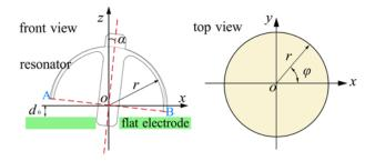
Fig. 1. The scheme of inclined assembly
