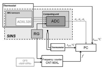
Fig. 1. Block diagram of the experimental stand
