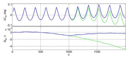
Fig. 5. Deviations of the LAN and LMST from the nominal values when passing the ascending node
