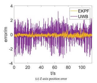
Fig. 12. Comparison of the position error of the indoor NLOS environment experiment
