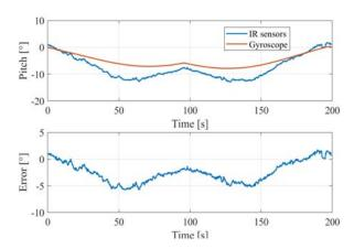
Fig. 11. Pitch angle calculated from the readings of IR sensors and gyroscopes
