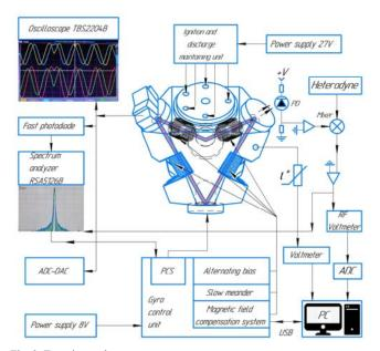
Fig. 3. Experimental setup.
