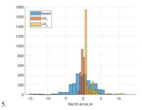
Fig. 4. Distribution of coordinate estimation errors along the North axis.
