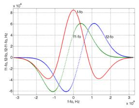
Fig. 2. Dependence of lasing frequency change of a mode of one circular polarization f1, of orthogonal polarization f2 and of their frequency difference on the cavity length detuning (frequency detuning) f=f1-f2.
