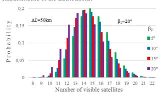
Fig. 2. Probability distribution of the number of visible satellites for two users with roll ( $\beta_1$ =20°,  $\Delta L$ =50 km)
