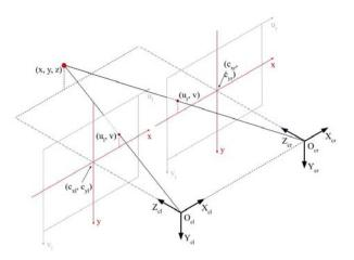
Fig. 1. Stereo camera model
