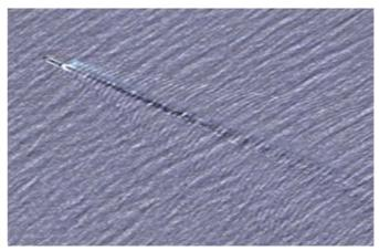
Fig. 1. Image of the wake of a cargo ship at the mouth of the Pearl River, China; received by the 'GF-1' satellite. The wake waves and the cuspid (pointed) waves framing them are clearly visible. The diverging Kelvin waves are faintly visible. Image resolution 8m. per pixel. Storm surge 5 points
