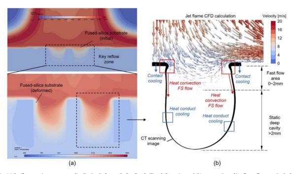
Fig. 2. (a) Jet flame static temperature distribution before and after fused silica deformation and (b) a separation of jet flame flow rate in the key silica reflow zone, calculated by a CFD simulation study
