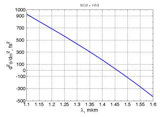
Fig. 14. Dependence of the group delay dispersion for a YAG: $Cr^{4+}$  gain medium of 2 cm long and a section of a quartz prism of 7.1 mm long on the lasing wavelength. Zero dispersion is observed at the wavelength of 1.46  $\mu$ m.
