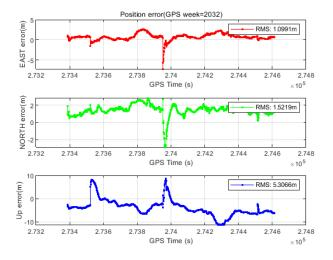
Fig. 3. The position errors in three directions with initial CKF
