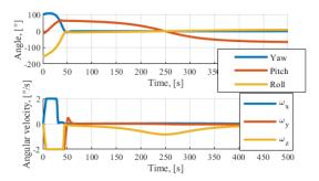
Fig. 3. Rotational motion of the satellite during simulation
