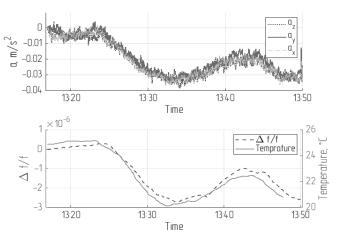
Fig. 3. Estimation of zero offset of thermally insulated accelerometers when the reference generator is heated
