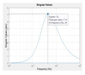
Fig. 3. Changes in the singular value of the closed system
