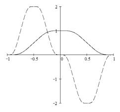
Fig. 1. Atomic function up(t) (solid line) and its first derivative (dashed line)
