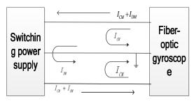
Fig. 4 Common mode (CM) noise and differential mode (DM) noise.
