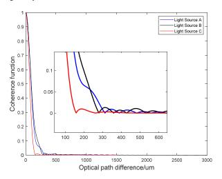
Fig. 6. Autocorrelation function of the ASE
