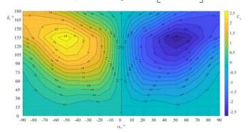
Fig. 3. Dependence of the pitching coefficient moment on the angle of attack and deflection angle for tail type 1
