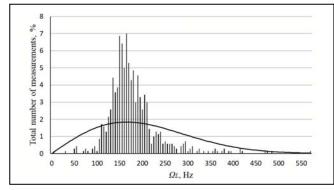
Fig. 3. Histogram of the distribution of the values of the lock-in threshold.
