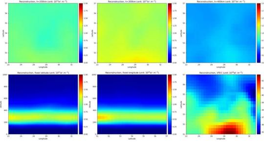
Fig. 3. Reconstruction of the electron concentration field before a geomagnetic storm.
