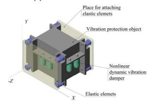
Fig. 1. Inertial instrument damping system.
