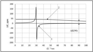
Fig. 2. A special view of the output characteristic of a laser gyroscope; type 1:  $S_1 = 0$ ; type 2:  $S_2 = 0$ .
