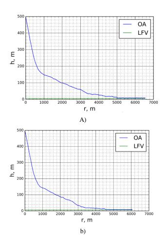
Fig. 3. Dependencies of heights of OA (OA – orbital aircraft) and LFV (low-flying vehicle) from passed distances
