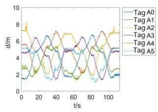
Fig. 11. UWB ranging data output for indoor NLOS environmental experiments
