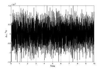
Fig. 4. Instability of the bench angular rate under simultaneous action of errors  $M_{\alpha}$ ,  $\Delta U_{in}$ ,  $M_{\beta}$ ,  $\Delta U_{fog}$  and  $M_{\phi}$  (in the case of ball bearing supports application).
