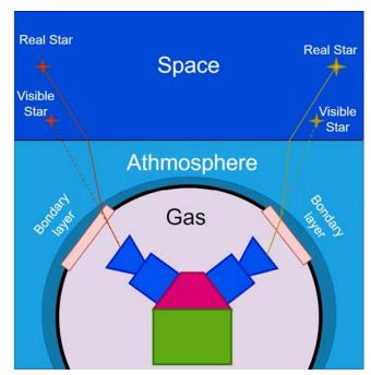
Fig.3. Refraction when observing stars in the atmospheric AINS.
