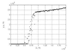
Fig. 3. Output frequency response with one longitudinal mode.
