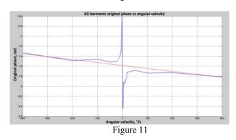
These diagrams demonstrate the presence of some constant value and a small linear dependence on input angular velocity. The original phase of the second  $b_2$  and third  $b_3$  harmonics strongly deviate from linearity at low angular velocities  $\omega$ <0°/s.
