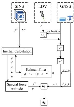
Fig. 2. Data processing procedure
