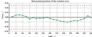
Fig.2 Graphs of rotary table errors after compensation.
