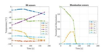
Fig. 14. Dependence of readings of IR sensors on solar illumination
