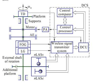
Fig. 1. Functional and kinematic diagram of the precision rotary test bench
