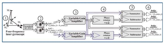
Fig. 1. Block diagram of separation of beat signals of counterpropagating waves of a Zeeman laser gyroscope according to orthogonal polarizations.
