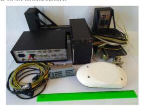
Fig. 1. Airborne collision avoidance system kit.
