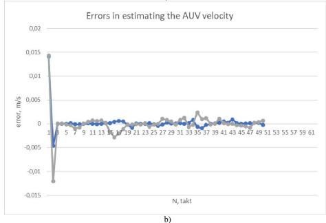
Fig. 2. Errors in estimating the AUV location (a) and velocity (b) (blue curve – for errors in measuring the course in the range of  $\pm$  0.1 degrees, gray curve – for errors in measuring the course in the range of  $\pm$  0.5 degrees).
