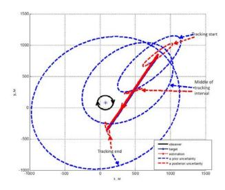
Fig. 1. Simulation of nonrecursive algorithm under the observer complete circulation
