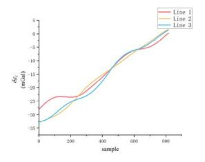
Fig. 5. Measurement results of gravity anomaly based on SINS/GNSS
