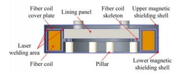
Fig. 5. Double-layer magnetic shielding structure
