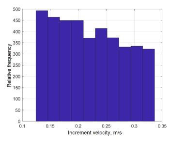
Fig. 2. Histogram of nanosatellite velocity increment values in the required direction in the absence of preliminary spin
