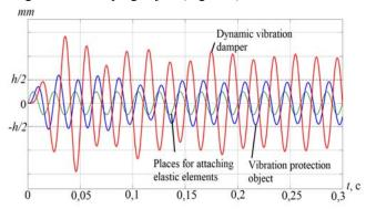
Fig. 5. Results of modeling the movements of the damping system at  $\Delta x > h/2$ .
