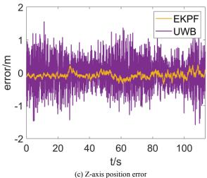
Fig. 9. Comparison of the position error of the indoor environment experiment
