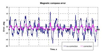
Fig. 4. Compass errors with the enabled and disabled correction system (heading  $K=0^{\rm o}$ ).
