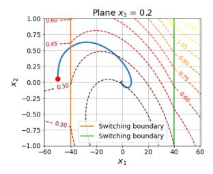
Fig. 1. Projections of the trajectory of a piecewise affine system and lines of the level of a piecewise quadratic Lyapunov function on a plane perpendicular to the axis  $\mathcal{X}_3$ .
