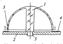
Fig. 1. Wave solid-state gyroscope with a flat node of electrodes: 1 - resonator; 2 - gyroscope base; 3 - metallized resonator surface; 4 - electrode; 5 - the junction of the resonator with the base
